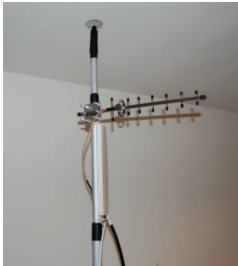
FIGURE 11.16 Expandable light pole used for temporary mounting and testing of Yagi and Patch antennas
