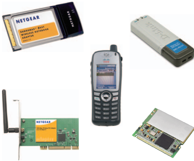
FIGURE 10.7 Client devices that are used with IEEE 802.11 wireless networking include external wireless client adapters, internal wireless client adapters, and voice over wireless LAN handsets
