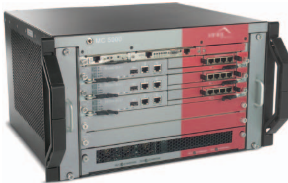
FIGURE 3.14 Meru MC 5000 large-scale enterprise wireless LAN controller
