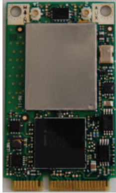
FIGURE 4.8 Intel 3945 IEEE 802.11a/b/g Full Mini-PCle adapter
