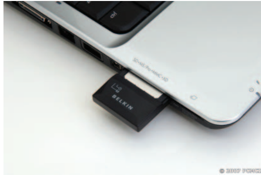
FIGURE 4.4 ExpressCard installed in a notebook computer
