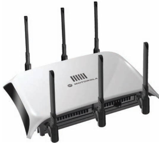
FIGURE 3.5 The Motorola AP 7131 IEEE 802.11n dual-band access point
