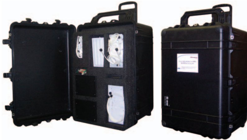
FIGURE 11.11 802.11n MIMO site survey kit from TerraWave Solutions contained in a durable and airline-approved transportable carrying case
