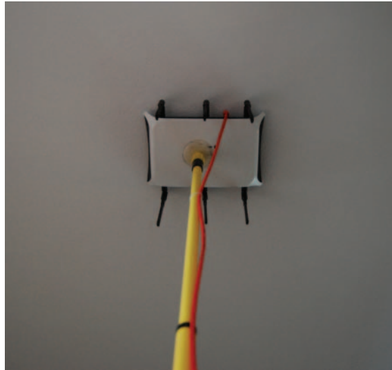
FIGURE 11.8 Access point temporarily mounted using an expandable light pole
