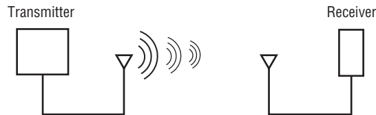
FIGURE 6.3 RF transmitter and receiver. In a wireless LAN, the transmitter and receiver could be an access point and client device.
